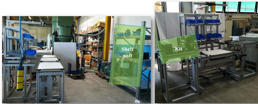
Figure 5 Assembly system configuration with line stocking (left) and kitting (right)
