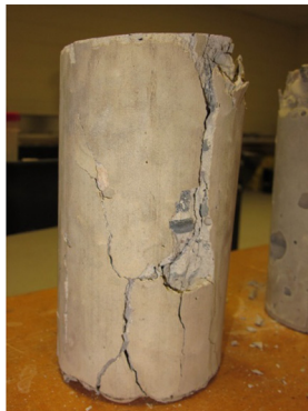
Type 3 Columnar vertical cracking through both ends, no well- formed cones
