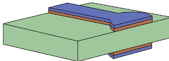
**Strip Resist:** Chemically remove the developed dry film resist.
