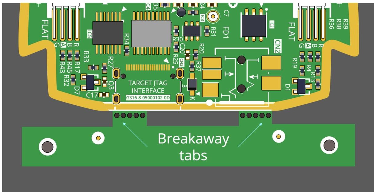
Figure 49 - Breakaway Tabs
