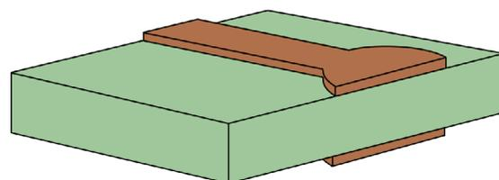
**Oxide Coating:** Chemically treat copper to roughen surface and improve adhesion to prepreg during the lamination cycle.
