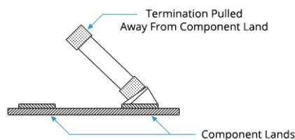
Figure 33: Termination Pulled Away from Component Pad Due to Poor Thermal Balance (Tombstoning)
