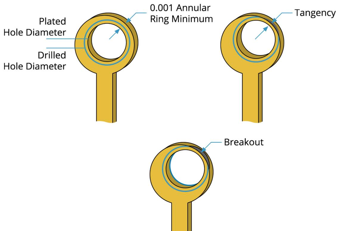
Figure 13 - Drilled and Plated Hole Diameters
