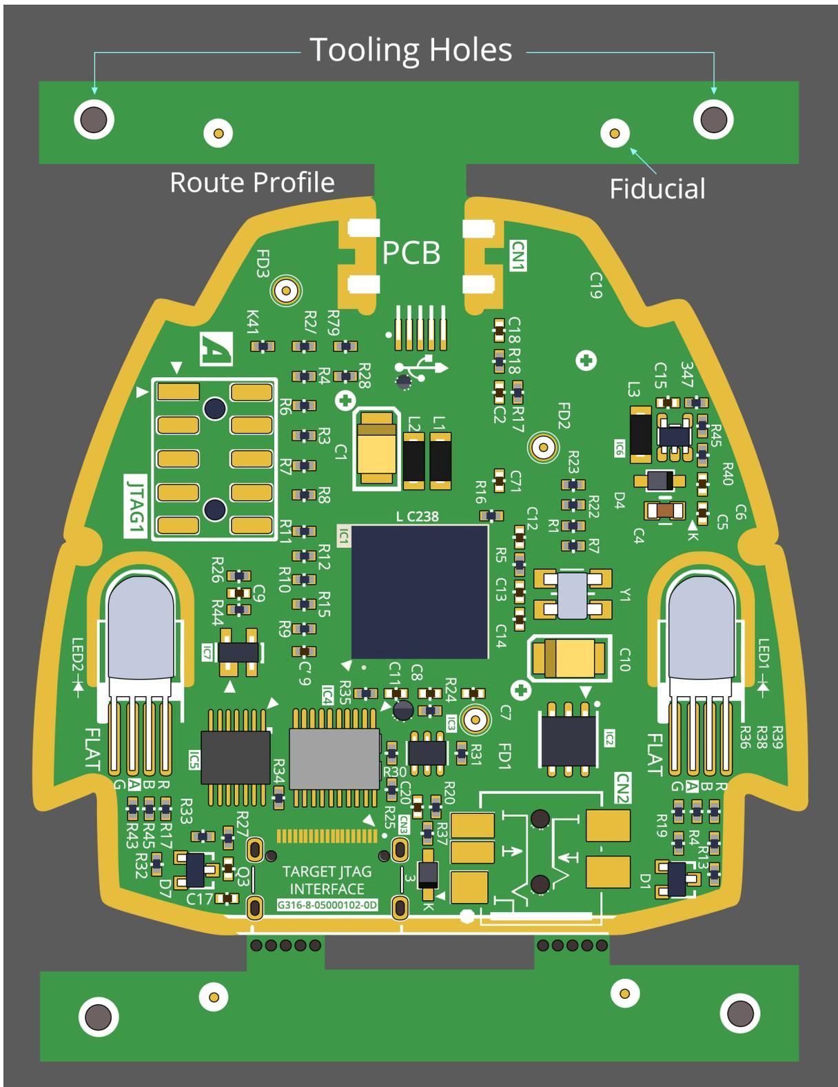
Figure 48 - Proper Tooling Hole Placement on a PCB
