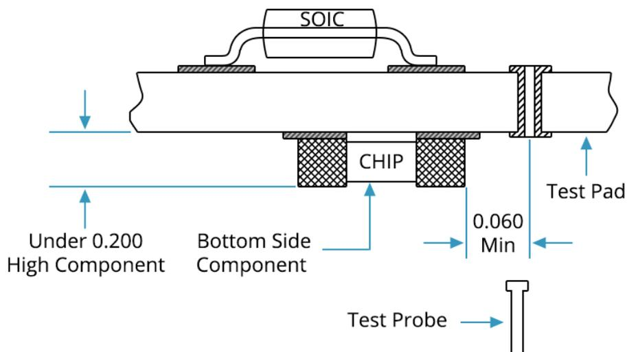
Figure 44 - Test Pad to Component Spacing for Components Under 0.200" Height
