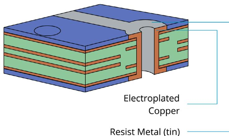
**Etch:** Copper is now removed from any area not covered by tin.
