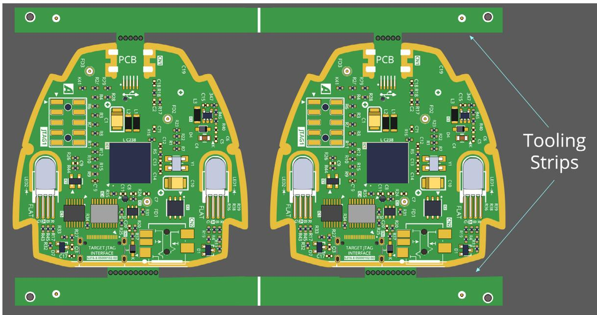
Figure 47 - Tooling Strips Along the Top and Bottom Edges of a PCB
