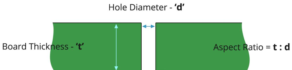
Figure 18 - Determining an Aspect Ratio for a PCB
