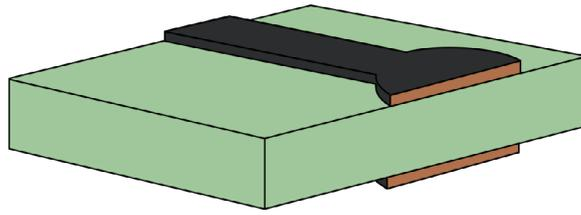
**Multilayer Lamination:** Copper foil, prepreg (multilayer glue), and cores are bonded together under heat and pressure.
