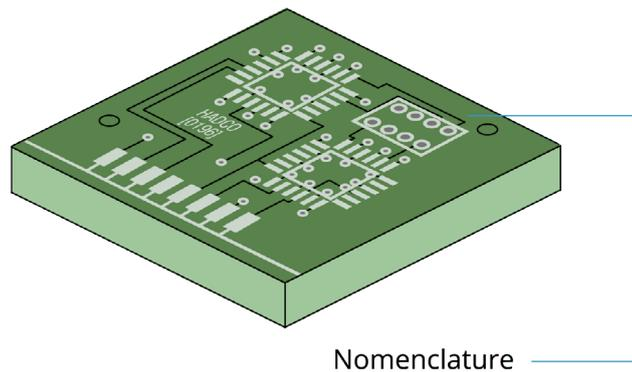
**Fabrication and Routing:** Board is cut to size (a.k.a routing, scoring, punching, or profiling). Slots and chamfers are also added during this step.
