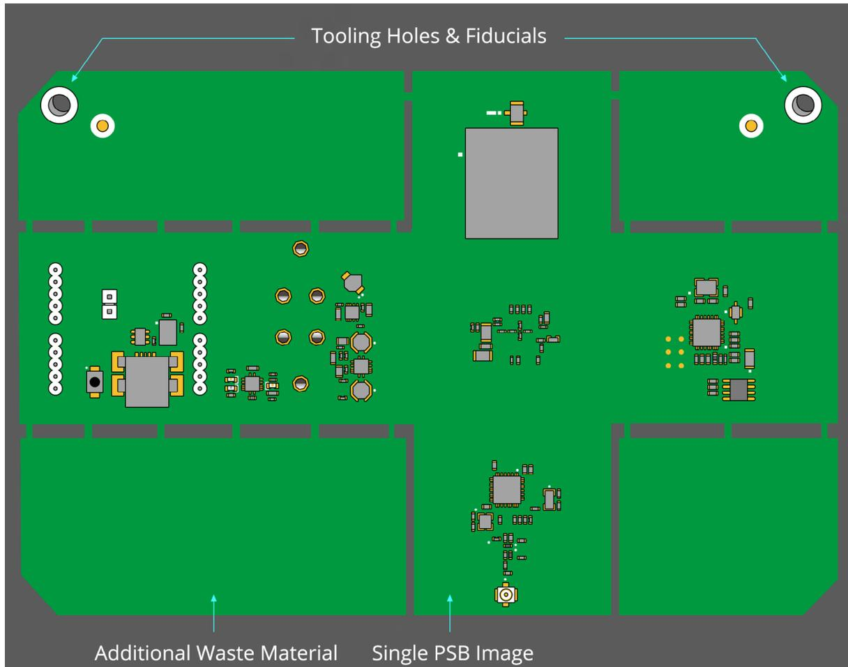
Figure 52 - Irregular Board with Infill Panels
