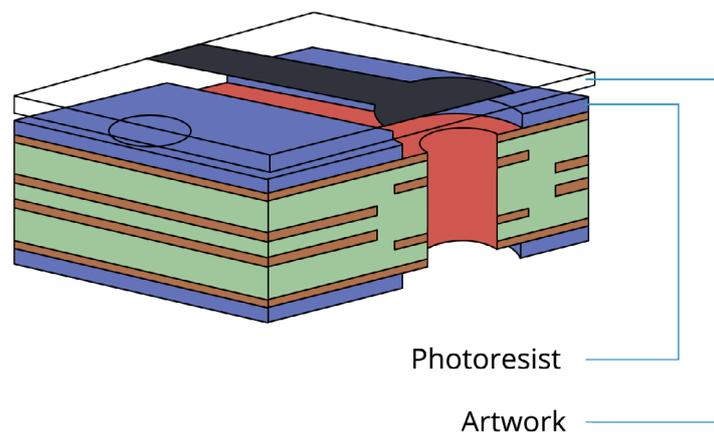
**Copper Pattern Plate (electroplating):** Additional copper (as well as tin) is electrically plated into the exposed electroless copper surfaces, as well as tin.
