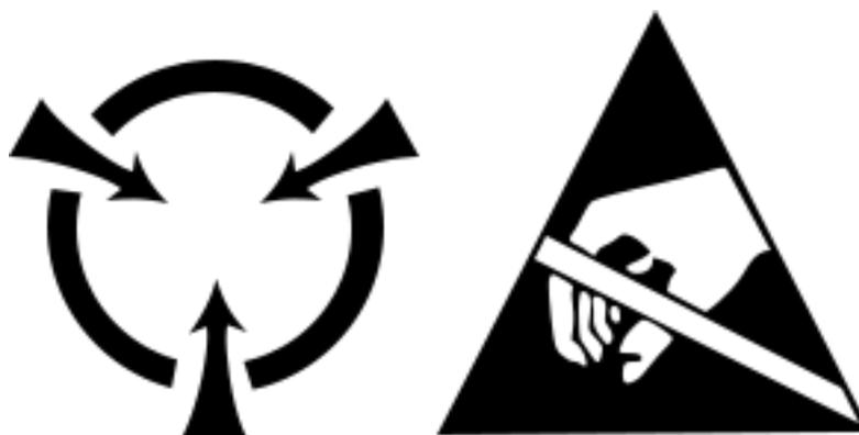
Figure 80 - Electrostatic Discharge Markings
