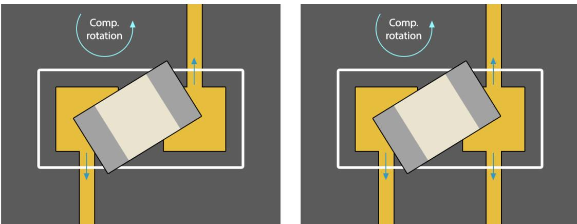
Figure 26 - Connecting Traces to Component Lands When Using Soldermask
