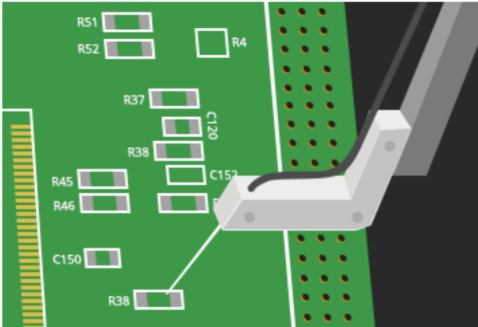
Figure 84 - Floating Probe
