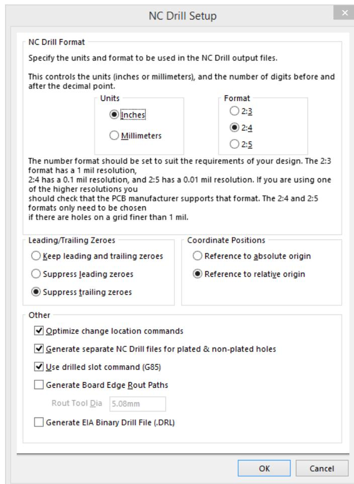
Figure 81 - NC Drill File Setup
