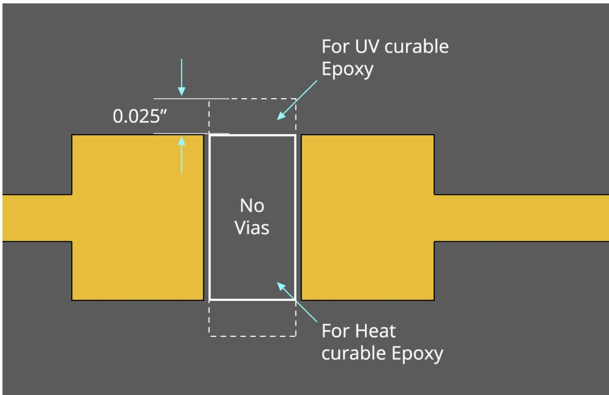
Figure 20 - Via Clearance Guidelines for Wave Soldering
