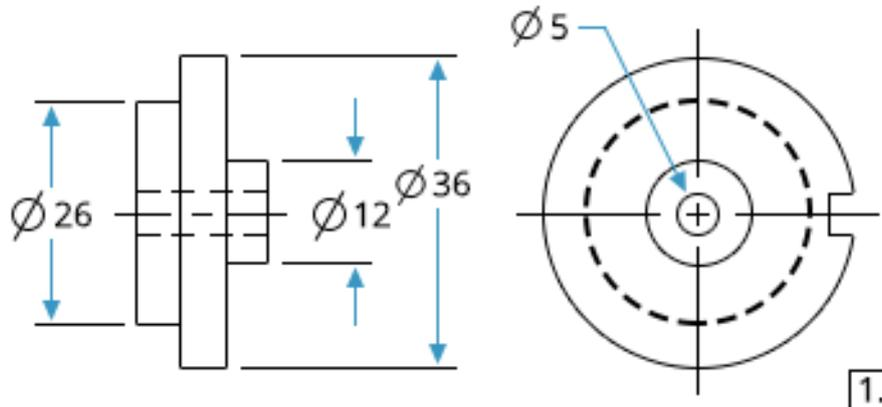
Figure 69 - Dimensioning Holes from a Side View
